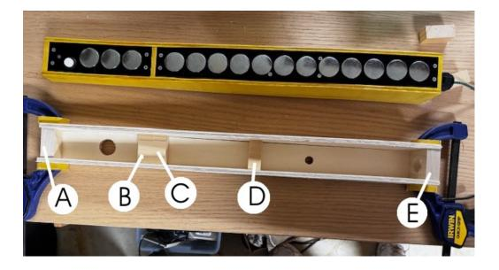
(E) <u>right end block</u> should be flush with the rightmost edges of the side panels with the bottom pressed against the upper surface of the bottom panel and the top about 1/8 of an inch below the upper edge of the side panels (this will provide a recess for the plastic button panels).
