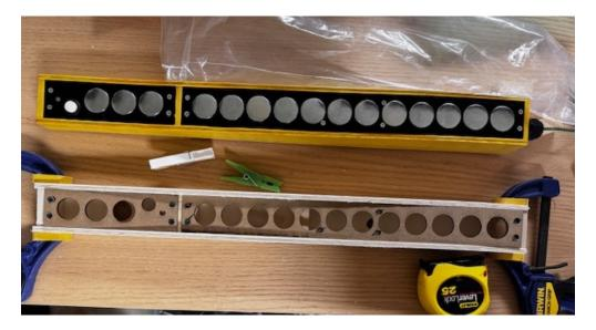
(f) Glue everything together and clamp. *Make sure that the bottom panel is flush with the bottom edges of the side panel*. I used wood clamps but it may be possible to do this with weights and rubber bands.
