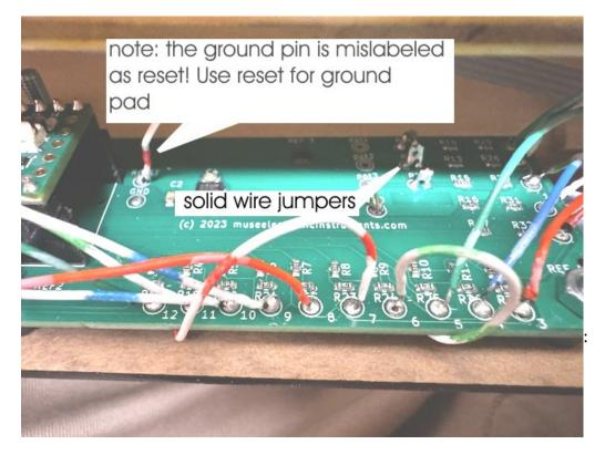
(g) Fish the USB cable through the strain relief and connect it to the Teensy and connect the Teensy to the print circuit boards so that the USB connector on the Teensy is close to the thick end of the housing.
