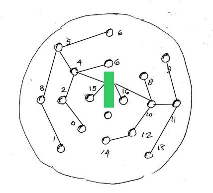
(q) Make similar connections using the red jumpers to connect each optical sensor to a 3.3 V pin on the printed circuit board. Any of the 3.3 V pins are acceptable. You can use the same pattern (it will probably keep you from making mistakes) that you used for the ground connections placing the red connectors next to the black connectors to help you double check visually. It can get quite confusing so be methodical. Double check that red wires only go to 3.3 V pins.
