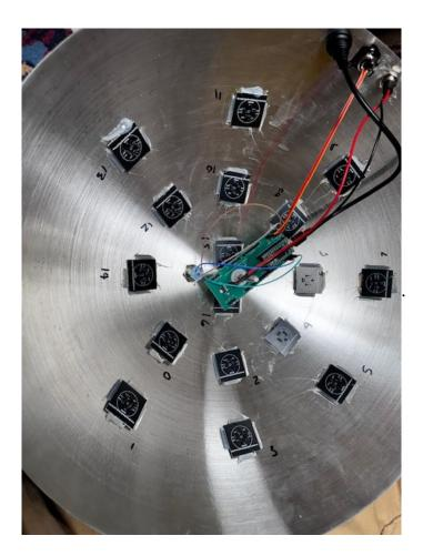
(p) Connect black jumpers from any of the ground pins and daisy chain the connections until you have connected all of the ground pins of all of the optical sensors. The exact order doesn't matter but here's a decent pattern. Triple check that these wires only connect to the ground pins labeled GND. Each optical sensor has multiple ground pins that are all interconnected so you can use any of them when connecting an optical sensor to another point or for making branches.
