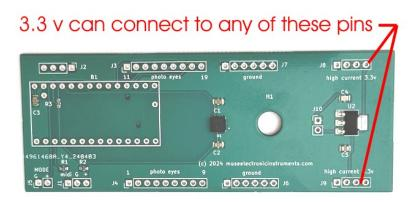
(r) Use the white jumper wires to connect an output from each optical sensor to the pin as on the printed circuit board as follows:
