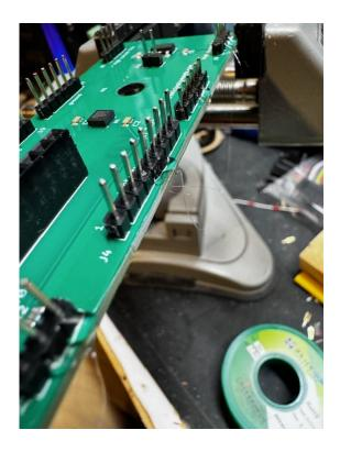
(j) Solder the pins on the Teensy (extending away from the side opposite side with the components) using the socket to line the pins up. For the moment, put away the Teensy for safekeeping in its static resistant bag
