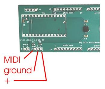
(o) Connect the pushbutton wires as follows:
