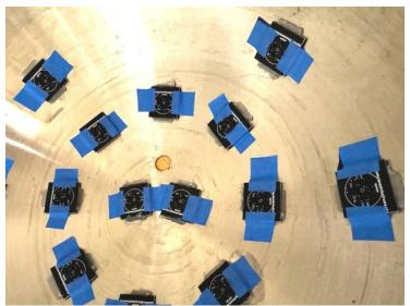
(c) Lay bead of silicon rubber on the exposed edges of each board joining that edge to the metal of the shell. Let everything cure and then carefully remove the tape and lay a bead of silicone rubber down on the remaining exposed edges so that all four edges are firmly attached to the inner surface of the shell
