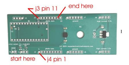
It gets quite complicated quickly so be careful. If you have a voltmeter, you can plug in the wall adapter at this time and check the voltages on each of the optical sensors
